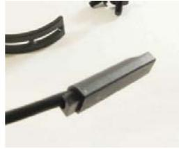
Fit the wedge to retain the sensor
