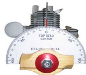
**For Adjustable Magnet Rings:** Turn magnet fixed ring anti clockwise. When you see the plug firing, stop and lock down the ring, the correct ignition timing is now set (28° ~30°). The plug will fire as the magnet passes slightly past the Hall Sensor, this is a normal condition.
