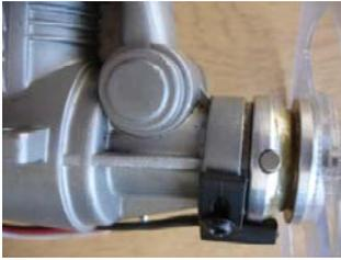
Generally the magnet is mounted in the prop driver and the sensor mounted to the crankcase. See below:
